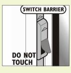
The switch barrier projecting from the locking mechanism, adjacent to the handle, is a safety device. It ensures that only one mode ('tilt' or 'turn') can be selected at any one time, by securing the handle into the selected mode, while the window is open.
